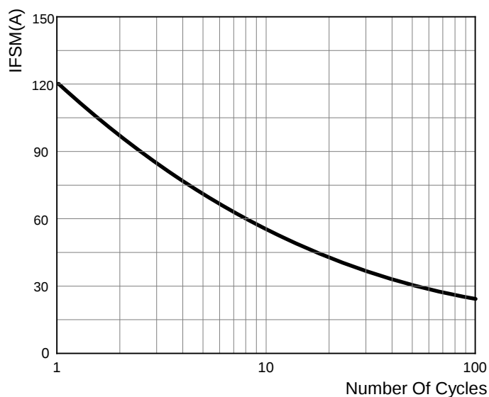
FIG.2: MAXIMUM NON-REPETITIVE FORWARD SURGE CURRENT
