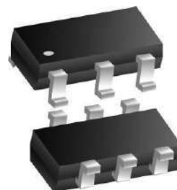
TSOP6 Pin Configuration
