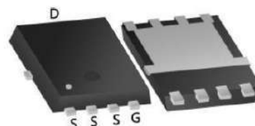
PRPAK3x3 Pin Configuration
