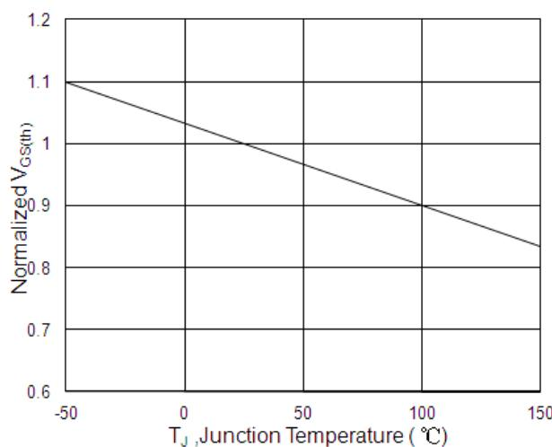
**Fig.5 Normalized V<sub>GS(th)</sub> vs T<sub>J</sub>**
