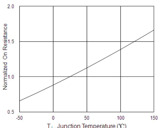
**Fig.6 Normalized R<sub>DSON</sub> vs T<sub>J</sub>**
