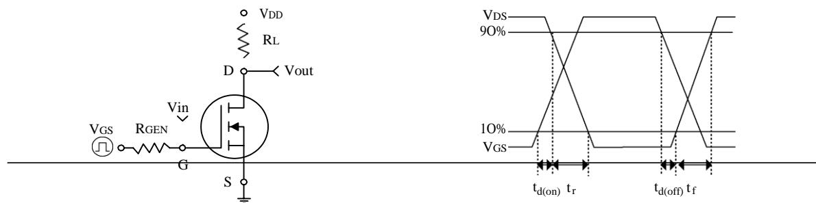
Switching Test Circuit and Switching Waveforms
